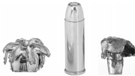
When bullets hit their targets, the soft lead deforms. The high-performance, expensive bullet on the left has “opened up” almost perfectly.
