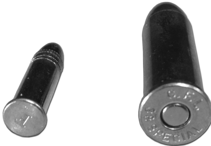
Rimfire vs. centerfire cartridges. At left is a .22 Long Rifle round, a rimfire cartridge. At right is a .38 Smith & Wesson Special round, a centerfire cartridge, seen from below. Note the telltale, circular primer cup that sits at the bottom of the centerfire cartridge's case head. The rimfire cartridge lacks this. Instead, it has a layer of priming compound (not visible) applied to the inside of the brass rim of the cartridge.
